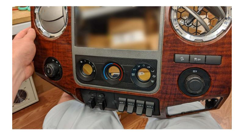
You will then need to attach the two mounting blocks to the HVAC control face using the included screws (m3x12mm) and epoxy the blocks into the dash bezel. It is important to make sure the HVAC controls are sitting as close to flush on the front of the dash bezel as possible:
