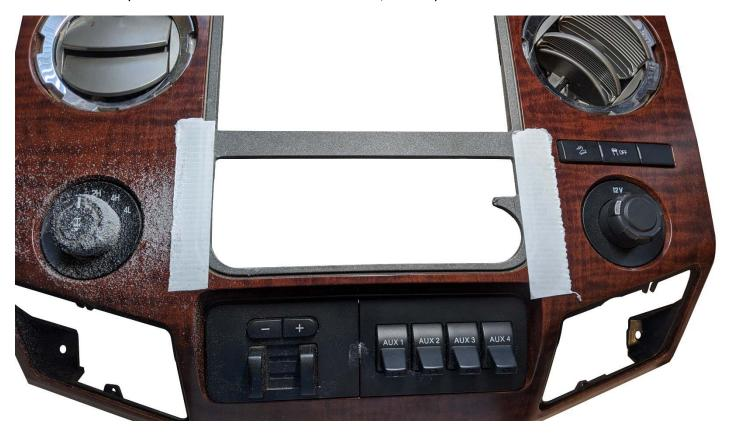
After removing the bar, carefully file the edges – this will be a finished edge, so take your time (we recommend using a hand file for the final work, not a Dremel):
